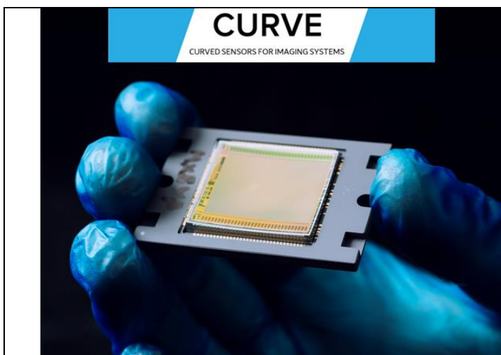
CURVE delivered the very first commercial curved sensor for a scientific application. This 12 MPixels model has a curvature radius of 150mm with a 5 microns regularity over the surface.
